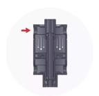
T1 (piston descending phase): internal transfer of the lubricant towards the expulsion chamber.
