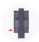
T2 (piston ascending phase): simultaneous aspiration and expulsion of the lubricant.
