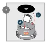
Insert new battery pack and seal. NOTE: the battery seal can be removed for 480cc cartridges.
