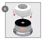
Replace cartridge on the MEMOLUB EPS series pump.
